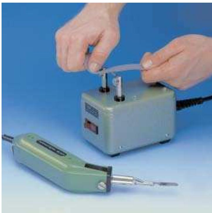
The handtool FG-HSG-0 is heated up in 6 - 8 seconds and lasts for about 20 minutes for short duration usage. The benchtool FG-TSG-00 is heated up in 15 seconds, suitable for continuous operation. The stationary cutting string has a 25mm working range and that is enough to cover all sizes of braided tubings.
